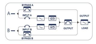
Under normal operating conditions, the INPUT (A) breaker, INPUT (B) breaker and OUTPUT breaker should be closed
